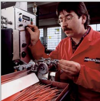
Heating wire winding machine
